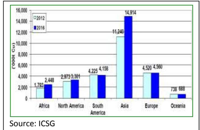
Meanwhile, Until 2016, world copper refinery capacity expected to grow by 4.6 Mt (18%) to 30 Mt. 3.6 Mt of the expansion expected to come from electrolytic refineries and almost 1 Mt from electrowinning capacity. The Supremacy of Asia continues over the other regions is likely to continue. Some growth in Africa and North America and the rest region is likely to remain practically unchanged.
